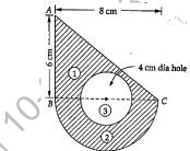
(b) Determine the centroid of the wire shown in below figure.
